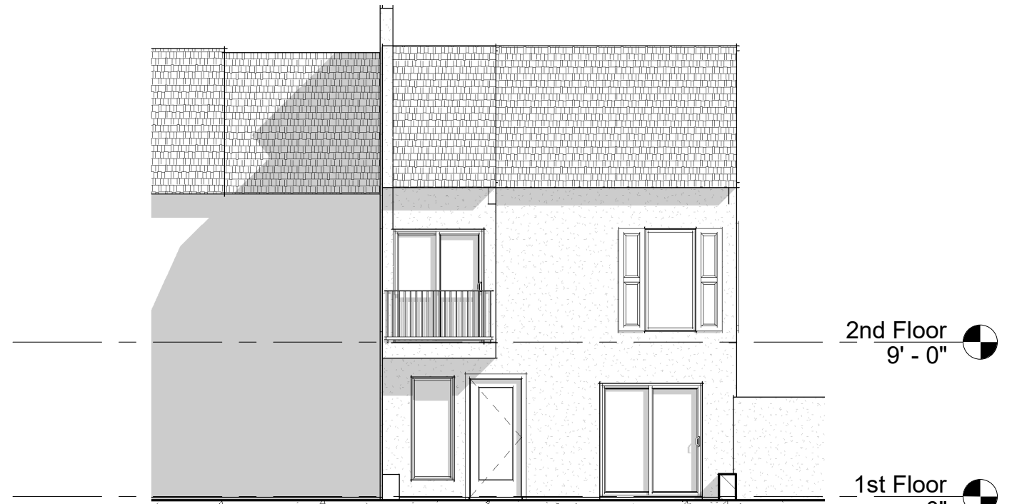
② Rear Elevation - Existing 1/8" = 1'-0"
