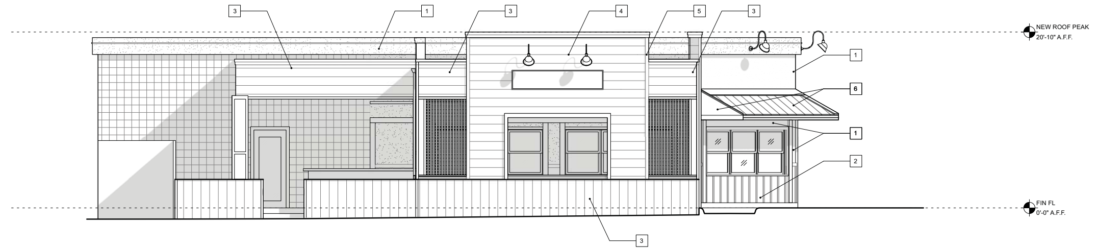
2 A202 WEST EXTERIOR ELEVATION - PROPOSED SCALE: 1/4" = 1'-0"
