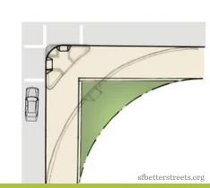
Slip lanes create multiple pedestrian conflict points and typically result in large turning radii. Removing slip lanes from intersections will create safer pedestrian crossings.
