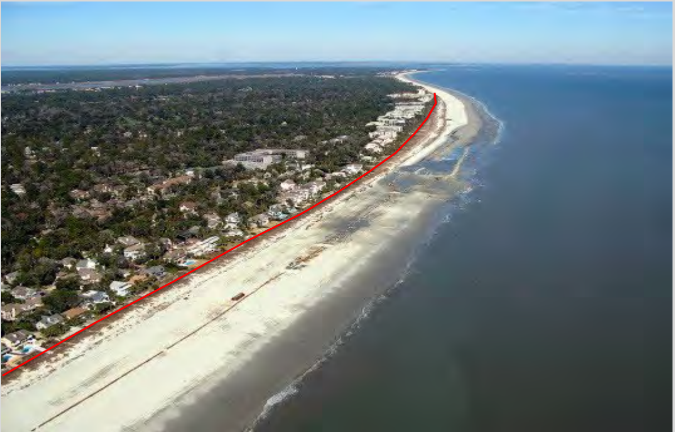
Figure 26: 2006/07 Project in Construction, with Pre-1990 Shoreline shown as Red Line.
