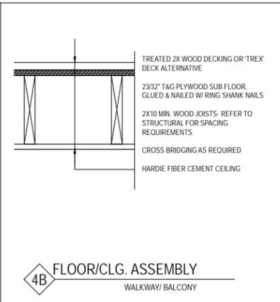
**CONSTRUCTION TYPICAL WALL, FLOOR / CEILING AND ROOF / CEILING TYPES**
