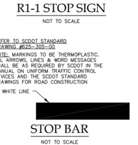
NOTE: MARKINGS TO BE THERMOPLASTIC. ALL ARROWS, LINES & WORD MESSAGES SHALL BE AS REQUIRED BY SCDOT IN THE MANUAL ON UNIFORM TRAFFIC CONTROL DEVICES AND THE SCDOT STANDARD DRAWINGS FOR ROAD CONSTRUCTION
