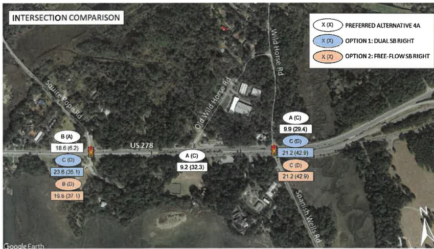
Figure 4— Intersection LOS Comparison
