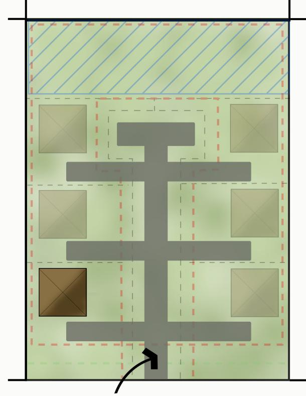
40' Right-of-Way required and all access must be installed at one time.
