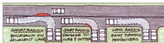
Intersection and Driveway Curb Radii
